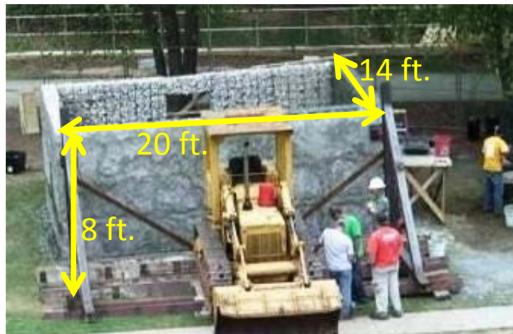
(e) Final look of the rubble house on SPSU campus. The picture was taken by the webcam before the static load testing.
