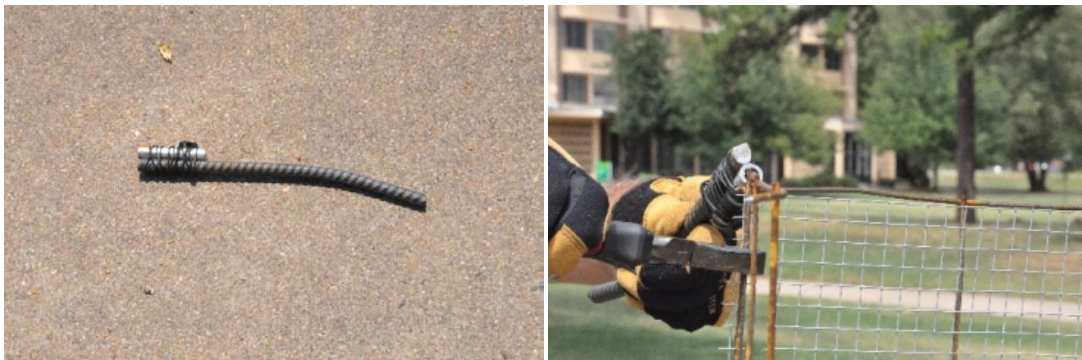
Figure 3 Bailey's tool used to bend wires.
