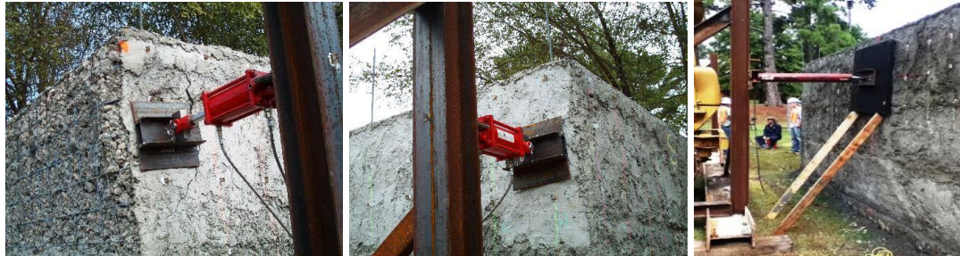
Test 1: In-plane loading (North Wall)
