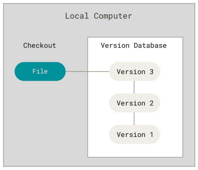
Figure 1. Local version control diagram
