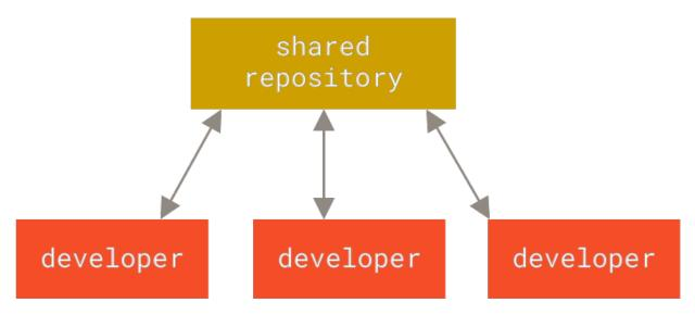
Figure 2. Centralized version control diagram
