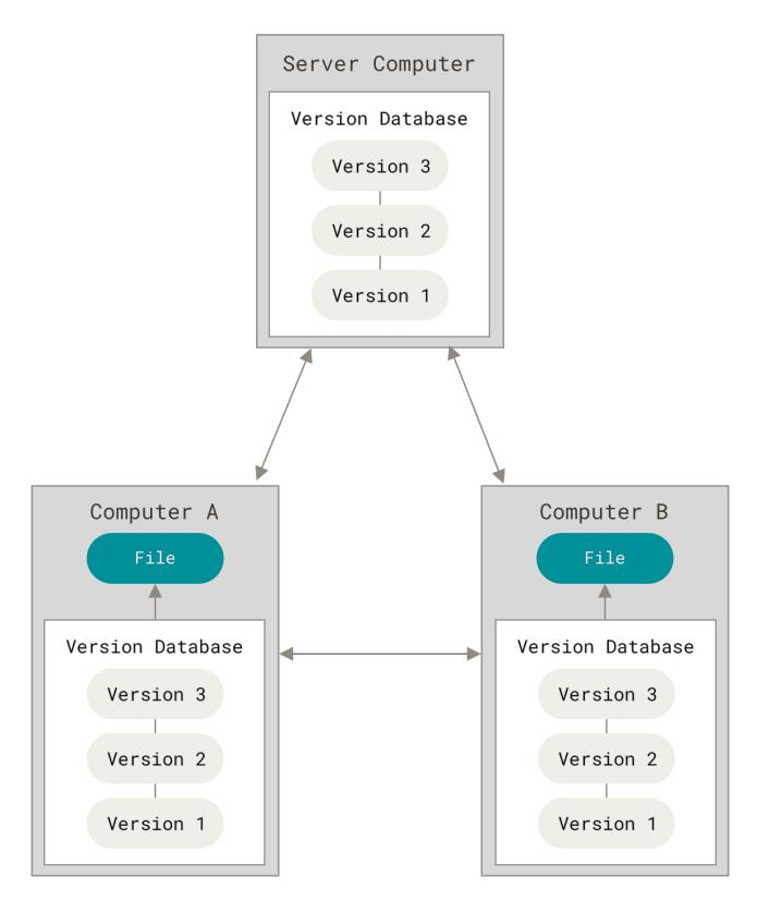
Figure 3. Distributed version control diagram
