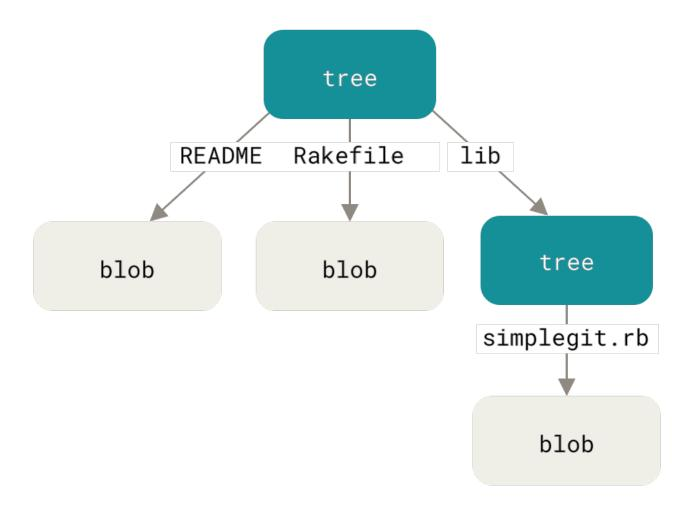
Figure 173. Simple version of the Git data model
