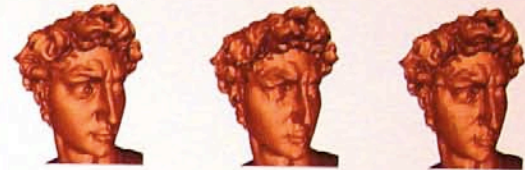
Figure 7. The original model is shown on the left. Simplified versions using uniform sampling (middle) and adaptive sampling (right). Both simplified models have the same number of polygons (approximately 1.5% of original polygons). Notice that the adaptive method preserves fine details.
